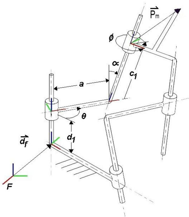
Figure 2. FORWARD KINEMATIC ANALYSIS
