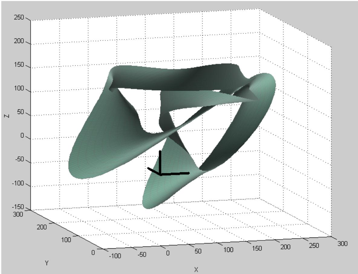
Figure 3. SPATIAL 4C CRANK-ROCKER COUPLER SURFACES
