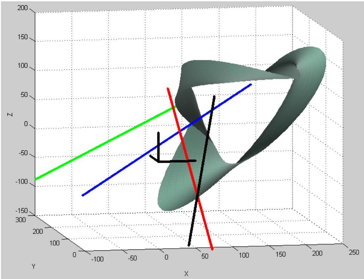
Figure 4. SPATIAL 4C CRANK-ROCKER: ONE COUPLER SURFACE WITH JOINT AXES
