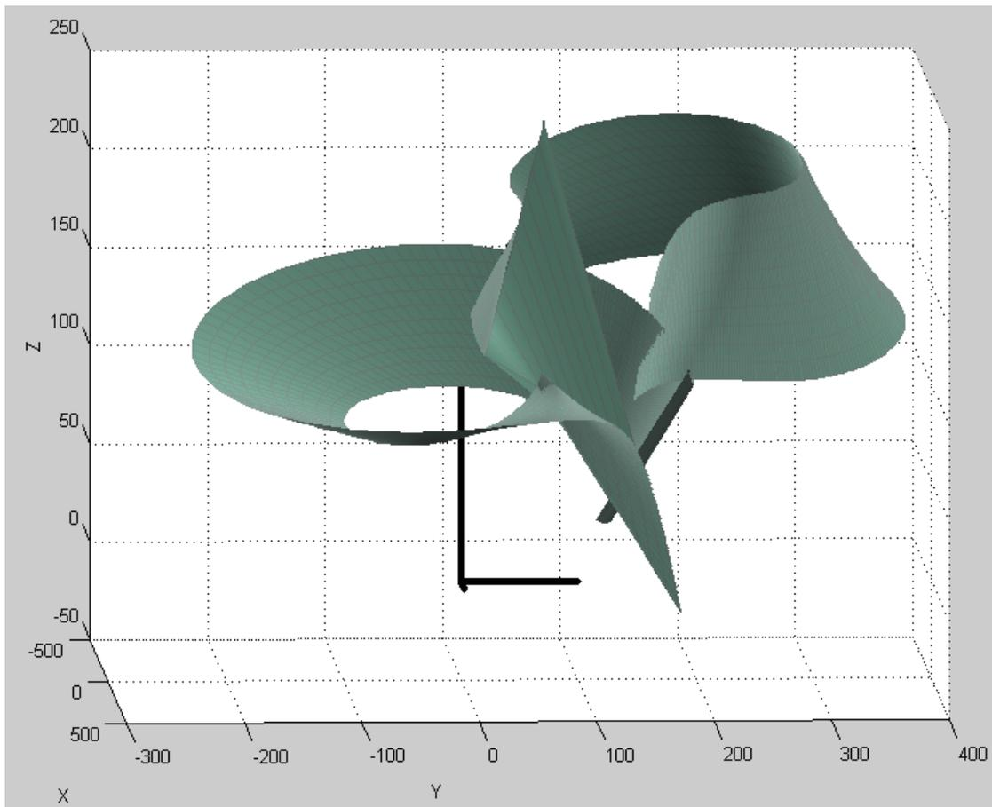
Figure 7. SPATIAL 4C DOUBLE-ROCKER COUPLER SURFACE: MODIFIED  $\theta$  RANGE
