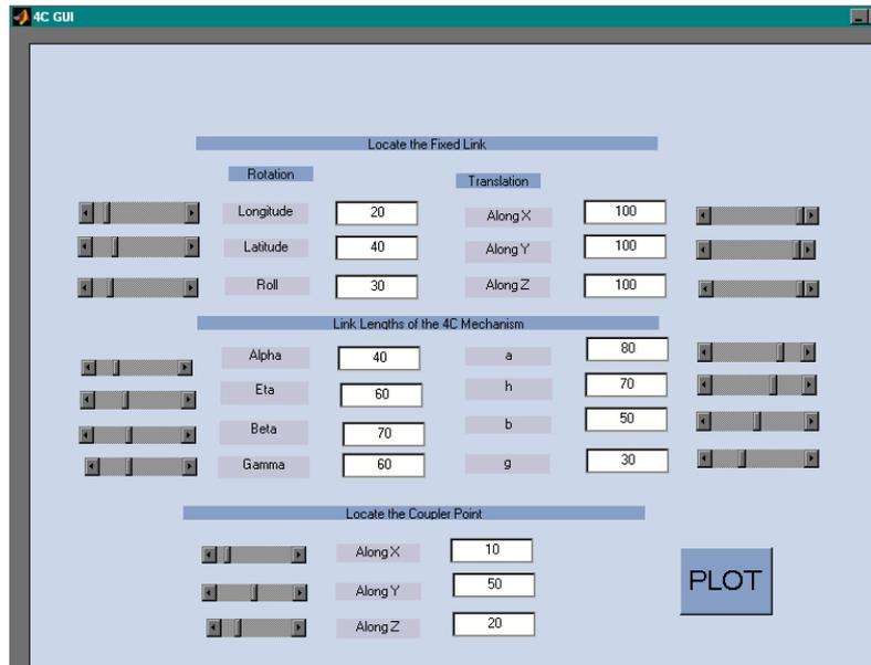
Figure 5. CRANK-ROCKER MECHANISM DATA AND USER INTERFACE
