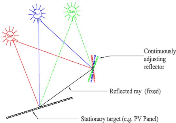
**FIG. 1: PROPOSED APPROACH: USE OF MIRROR-POSITIONING DEVICE (MPD).**
