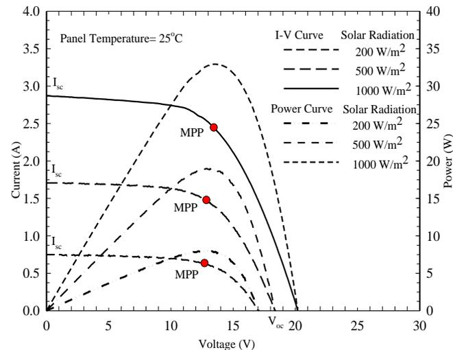
**FIG. 2: I-V CURVE AND POWER CURVE OF THE PHOTOVOLTAIC PANEL AT 25°C PANEL TEMPERATURE AND AT VARYING SOLAR RADIATION.**
