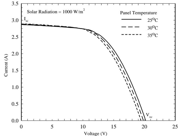
**FIG. 3: I-V CHARACTERISTICS OF THE PHOTOVOLTAIC PANEL AT DIFFERENT PANEL TEMPERATURES AND AT 1000 W/ M<sup>2</sup> SOLAR RADIATION.**
