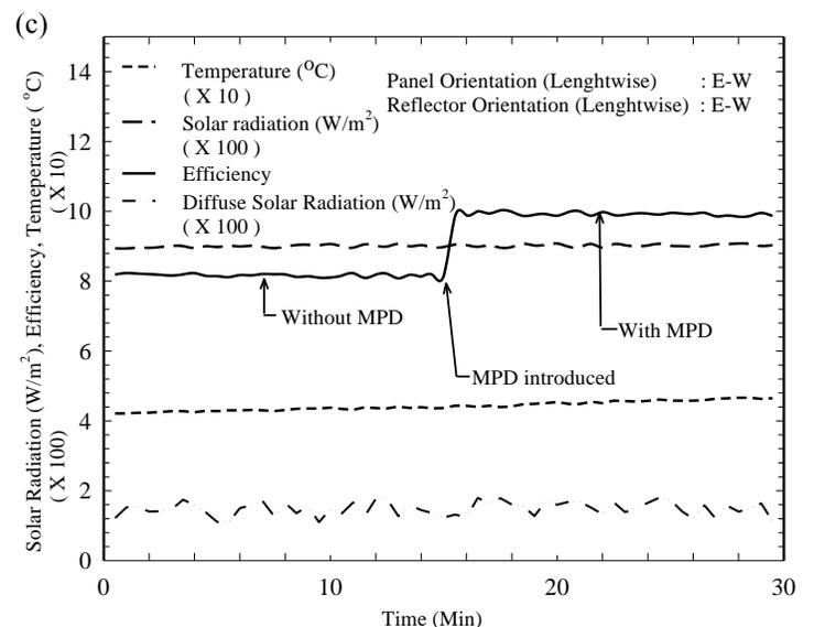
**FIG. 5: EFFICIENCY ENHANCEMENT DUE TO APPLICATION OF MIRROR POSITIONING DEVICE FOR DIFFERENT SOLAR RADIATION.**
