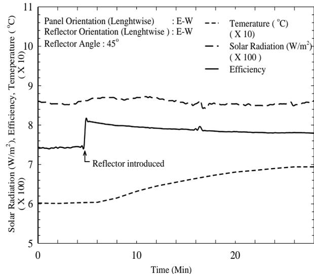
**FIG. 4: EFFECT OF STATIONARY REFLECTOR ON THE EFFICIENCY AND TEMPERATURE OF THE PHOTOVOLTAIC PANEL.**
