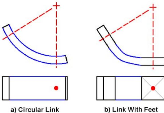
Figure 4. LINK GEOMETRY.
