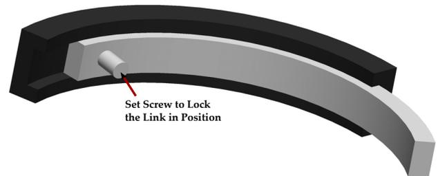
**FIGURE 17.** AN ADJUSTABLE SPHERICAL LINK (Hong & Erdman [1])
