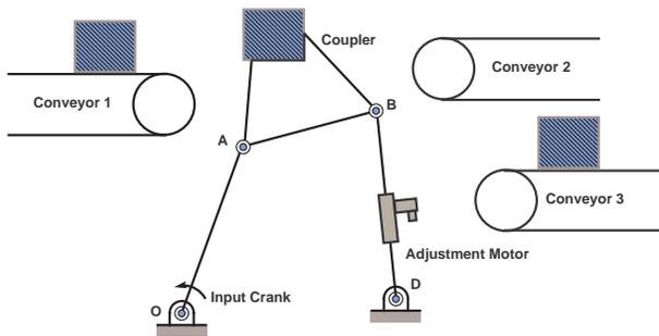
**FIGURE 3.** AN ADJUSTABLE PLANAR LINKAGE (Chuenchom and Kota [3]).
