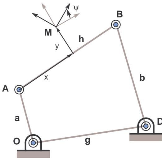
**FIGURE 6.** FOUR-BAR MECHANISM PARAMETERS.
