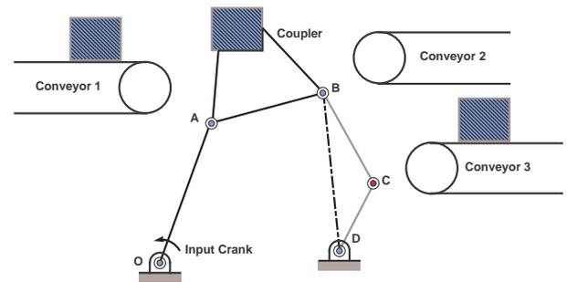
**FIGURE 4.** PROPOSED ALTERNATIVE DESIGN: USING A RMG.
