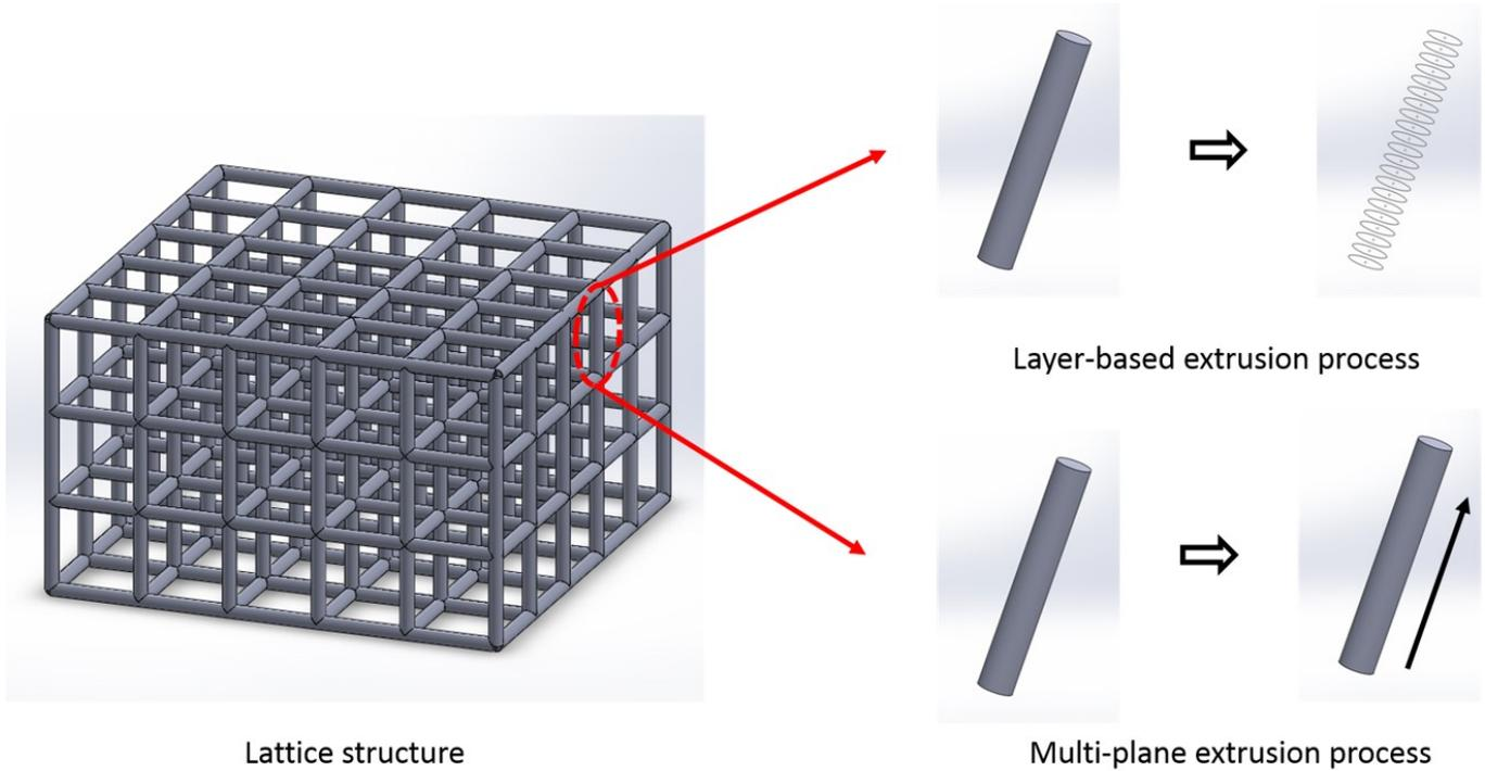
**FIGURE 1:** COMPARISON OF 3D LATTICE STRUCTURE FDM PRINTING BASED ON DIFFERENT APPROACHES.
