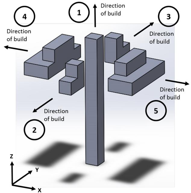
**FIGURE 6: BUILD DIRECTION SELECTION.**
