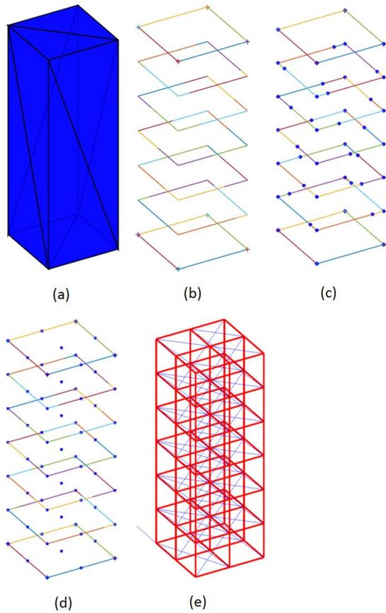
**FIGURE 7: STEPS PROCESS FOR 3D LATTICE GENERATOR.**
