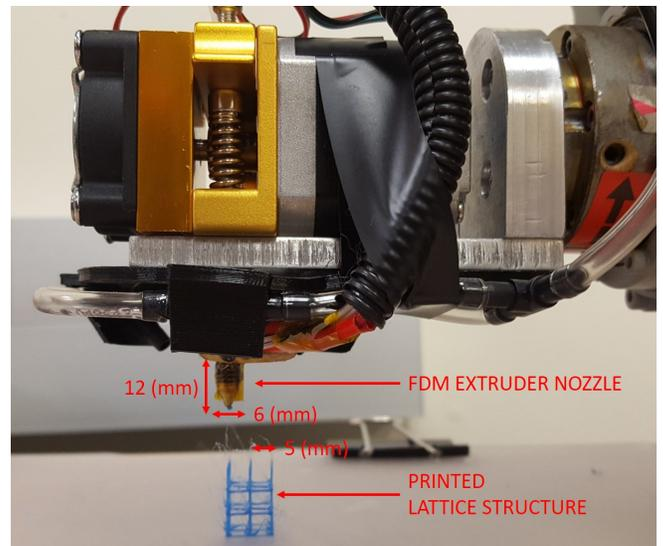
**FIGURE 9: FDM NOZZLE CLEARANCE.**
