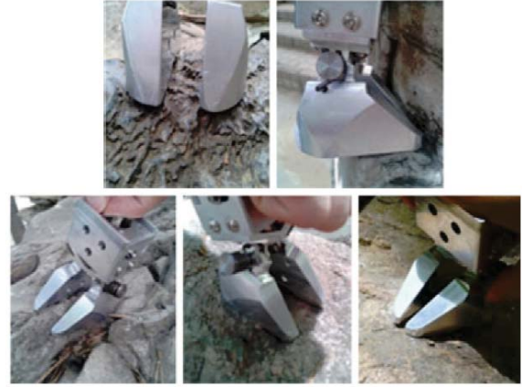
Figure 7. Prototype of the Bioinc Foot Inspired by Blue Sheep [7]
