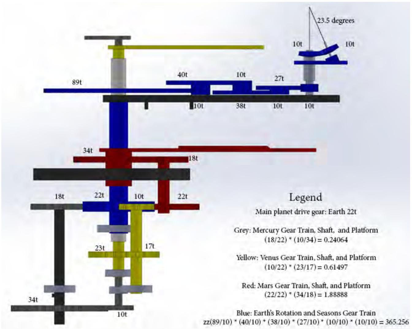
Figure 3: The gears, their teeth numbers, and how the gear train system is connected
