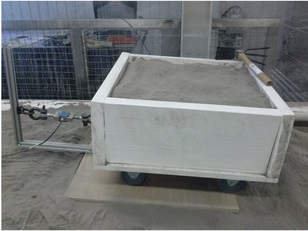
Figure 5. Test Bin with Load-Cell
