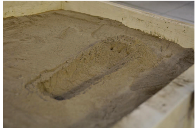
Figure 8. Excavated Path created by 3 Rod Anchor.
