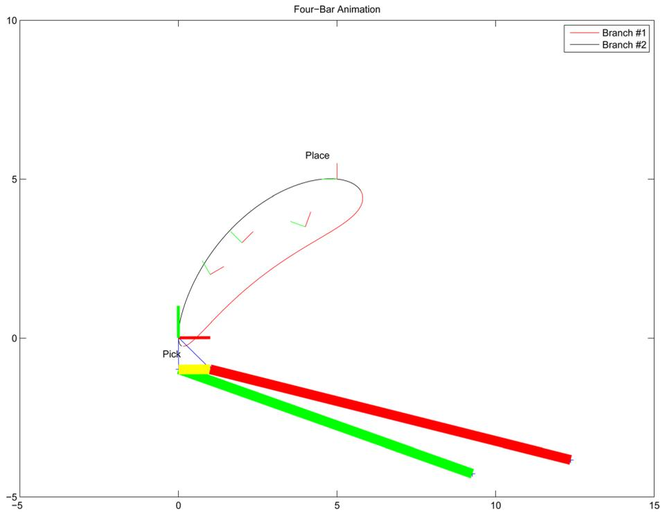
Fig. 7 The mechanism shown in the pick position
