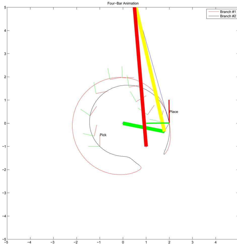
Fig. 12 The mechanism shown in the place position
