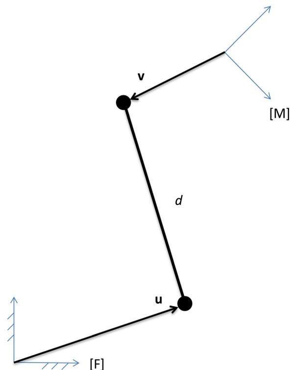
Fig. 1 Planar RR dyad geometry and nomenclature
