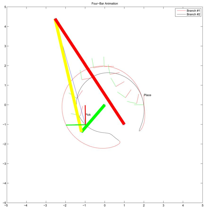
**Fig. 11 The mechanism shown in the pick position**
